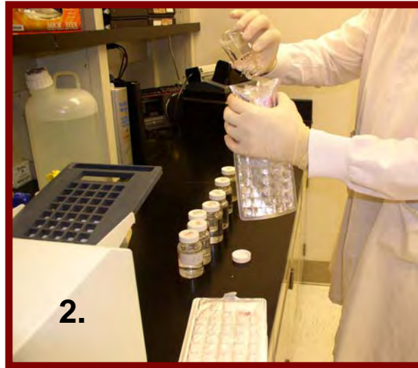
2. Sample poured into Quantitray
