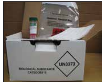
Biological Substance, Category B Box with 95kPa bag and Air Pillows
