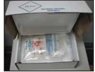
Place sample bag on top of frozen freezer block and replace styrofoam lid
